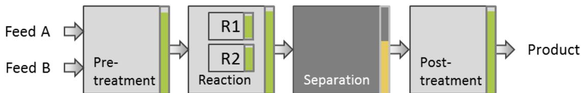
**Figure 2: Overall efficiency indicators in plant structure diagram.**
