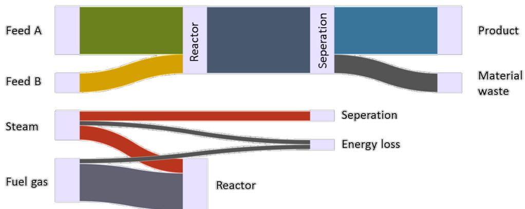
**Figure 4: Sankey diagram for materials (top) and energy (bottom).**
