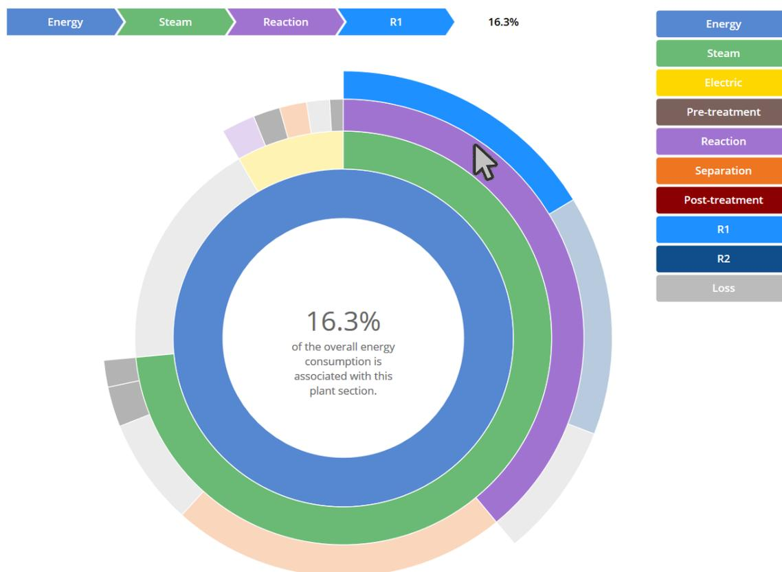
**Figure 3: Sunburst diagram for the energy consumption by plant section.**
