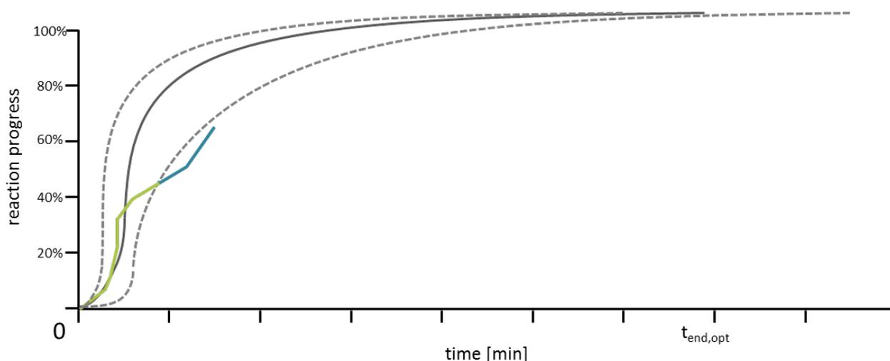
**Figure 11: Real-time trajectory plot of the reaction progress of a batch reaction phase. Optimal trajectory (solid gray line), normal operation range (dashed gray line) and the current trajectory (green/ blue line).**
