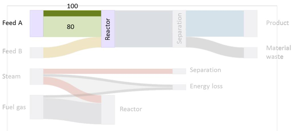
**Figure 5: Sankey diagram with highlighted raw material feed A with a measured flowrate of 100 and a theoretical minimum of 80 to produce the same amount of product.**
