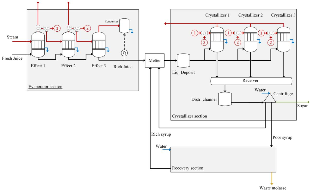
**Figure 5. Flowsheet of the sugar plant for the production of food-grade sugar from sugar beets**
