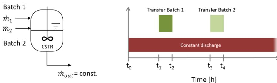
**Figure 3: Buffer tank between batch and continuously operated section (left), timing of transfer operations to and from buffer tank (right)**
