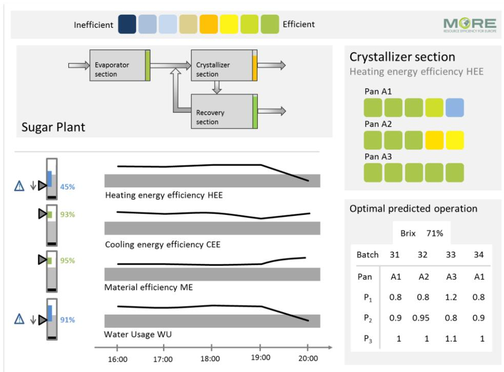
**Figure 7: Dashboard concept of the sugar plant with optimization-based decision support.**
