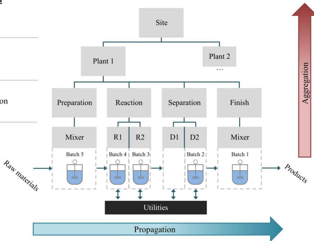
**Figure 1: Hierarchical structure of a batch production site on four levels, with the reaction stages R1, R2 and the distillation stages D1, D2.**
