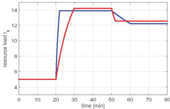
**Figure 4: Resource utilization  $r_k$  per product in the buffer tank for different transfer times for the same two batches with different efficiencies**
